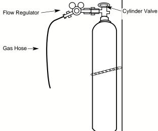
With the cylinder securely installed, remove the cylinder cap. Stand to one side away from the outlet and open the cylinder valve very slightly for an instant. This blows away any dust or dirt which may have accumulated in the valve outlet.
